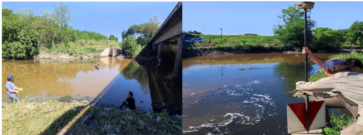
Figure 13: Measurement of points in water with kayak (left) and measurement of points on land with quadrant (right).
