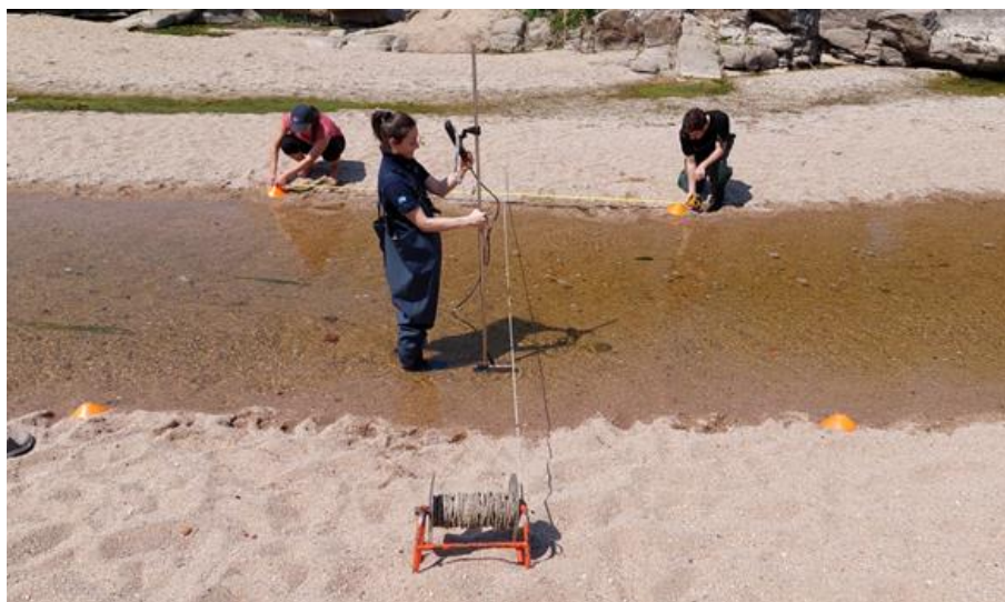
Figure 6: Picture of the field test conducted by INA in Córdoba, using the draft of LSPIV measurement guidelines
