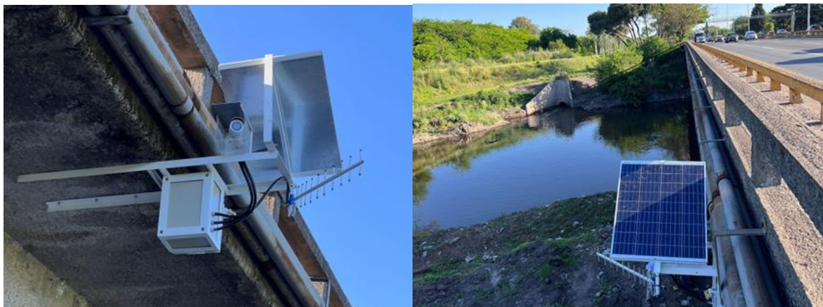
Figure 11: Installed fixed LSPIV station (left) and panoramic view from the installation point (right)
