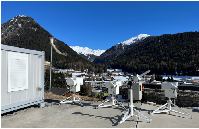
Figure 3. Three generations of total ozone column (TOC) instruments at Davos. The container on the left contains three automated Dobson spectrometers (first generation of TOC instruments). Three Brewer spectrometers (second generation) can be seen at the back. In the centre at the front: the new BTS-Solar instrument (third generation).
