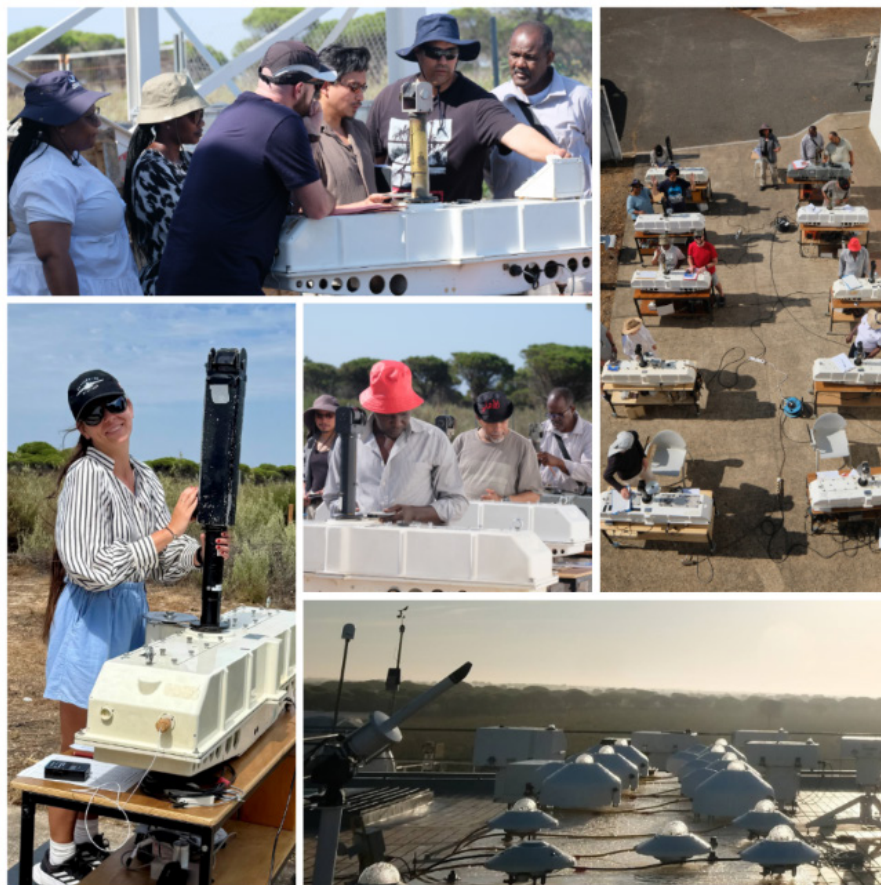
Figure 5. Top left: On-site, hands-on instruction during intercomparison campaigns is essential for teaching key techniques and refreshing operational procedures. Top right: Ten Dobsons, including the European standard. Bottom right: Brewers, a BTS-Solar spectrometer and other instruments measuring UV and ozone alongside the Dobsons. Bottom left: Dobson #073, one of the British Antarctic Survey (BAS) instruments that contributed to the discovery of the ozone hole (Farman et al., 1985), was flown in from Antarctica for maintenance in Germany and calibration in Spain, operated here by S. Kucieba (BAS). Centre: Instruments from Uganda (#056), Egypt (#069), and Algeria (#011) – one of the oldest Dobsons still operating, built around 1932 – also took part in the campaign.
